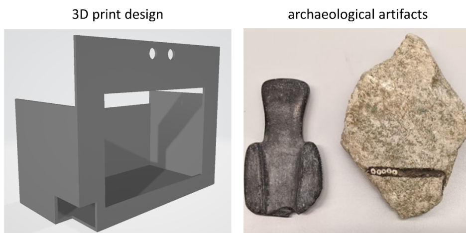
Figure 47. Example of 3D printed sample holder for unique samples.
