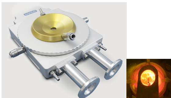
Figure 39. Linkam furnace (left) and its heated sample compartment (right) with a calibration thermocouple placed at the center of the sample. The furnace can be operated in the range RT-1100°C in a protective atmosphere.
