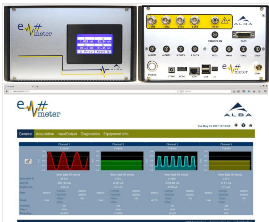
Figure 14. Front and rear view and web-based GUI of the Em#.
