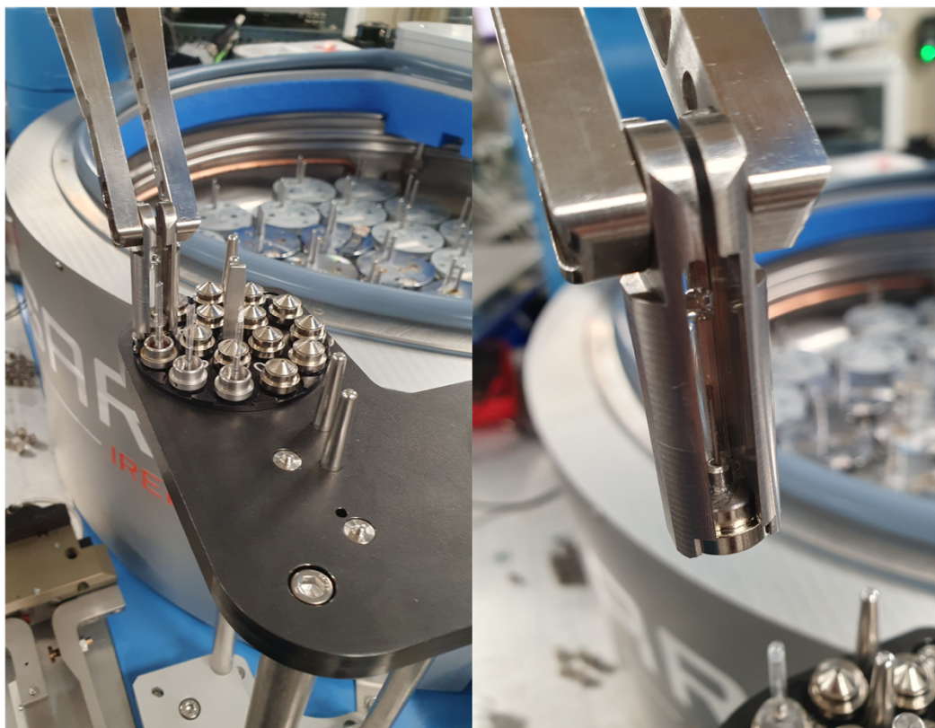
Figure 2.4: ISARA hot tool with single gripper. Note how the gripper picks up the sample at the base, leaving plenty of space to avoid damaging the attached capillary.
