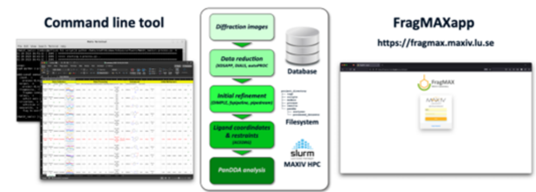
Figure 2.33 Automated data analysis options at FragMAX. The platform offers a command line processing toolbox which is usually launched by FragMAX staff, as well as an interactive web application (FragMAXapp) that can be run by users.
