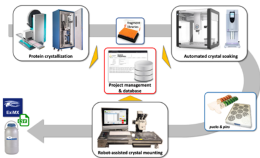
Figure 2.32 Schematic of the FragMAX crystal preparation workflow.
