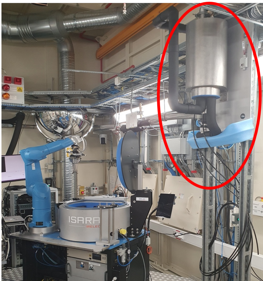
Figure 2.5: Phase separator (highlighted in red) installed by the ISARA dewar.
